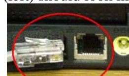
Network port on a computer
